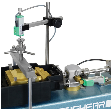
Detail of shear box housing made of high resistance techno-polymeric material and digital measurements.
